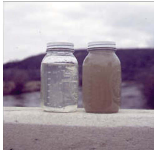
The water in the clear jar on the left has about 10 mg/l of suspended sediment, whereas the jar on the right contains about 500 mg/l of sediment
