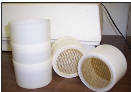
Soil sieves can be used to separate out different sized particles of soil.
