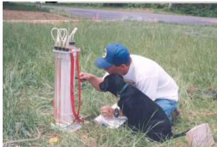
A Soil Scientist is recording readings from a Constant Head Permeameter, used to measure saturated hydraulic conductivity ( $K_{sat}$ ).
